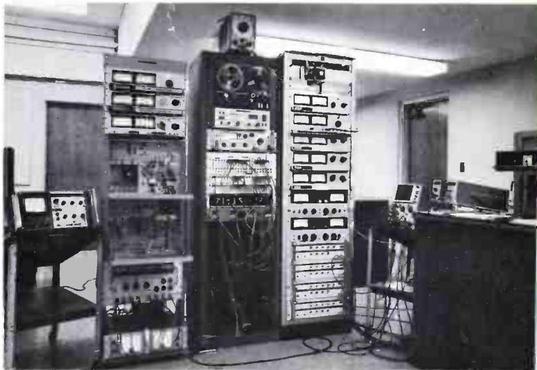
Four-channel signal generating equipment is set up in center and right racks in this laboratory at the College of San Mateo, California. In left rack is the Cooper-UMX system, undergoing tests.
