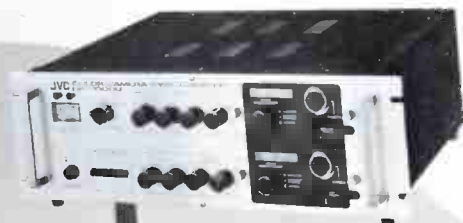
GK-2000U sync coupler weighs 10 lbs. with 2 CCU's. Approx. 14" wide, 14" deep, 6" high.
